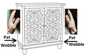
Pat and wobble the sides of frame couple times until the doors are aligned and leveled. Then tighten the #1 bolts
