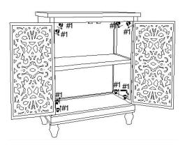
Open the doors, loosen the #1 bolt a little bit, then close the doors.
