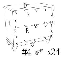
After doors are perfectly aligned, assemble the back panel and tighten the #4 screws.
