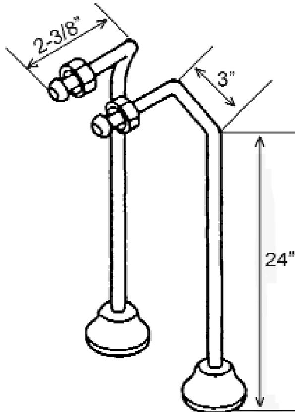
**Use on concrete floors requires special installation. We recommend using a plumbing professional.**
