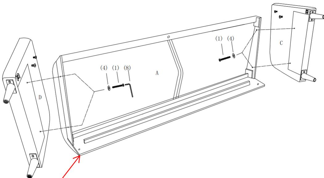
Notice: This is the front panel! Do not assemble in wrong direction.
