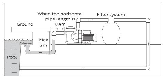
Note: The dry pipe before the pump inlet must not exceed a total length of 2.4 meters.
