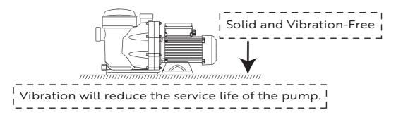
2. Fill the pump with water before starting. Do not run pump dry. Water acts as a coolant and lubricant for the mechanical shaft seal. Running pump dry may damage seals, causing leakage, flooding, and void warranty.
