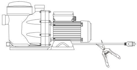
2. Peel off the black cable skin to reveal the 3 wires inside, strip each cable by 2/3 inch with a wire stripper, then strip the insulation to reveal 1/5 inch copper wire. Prepare the wire extension of the pump and repeat the above steps.
