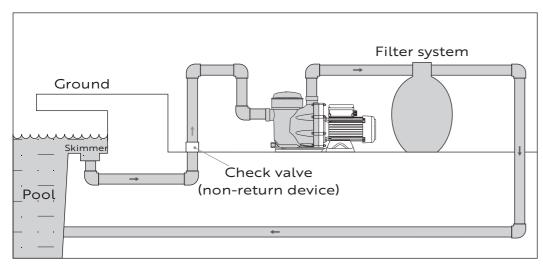
7. Above-Ground Pool: The pump inlet is positioned below the water surface, enabling direct flow of water from the pool into the pump.
