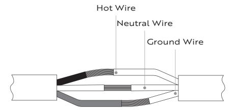
4. Winding the waterproof electrical tape around the butt splice connections of the three strands of wire.
