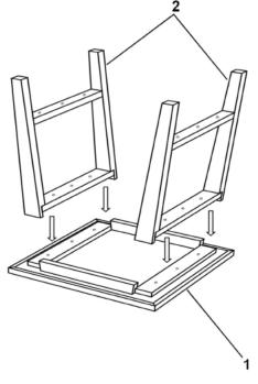
STEP# 2: Tighten the bolts to lock the legs as shown below.
