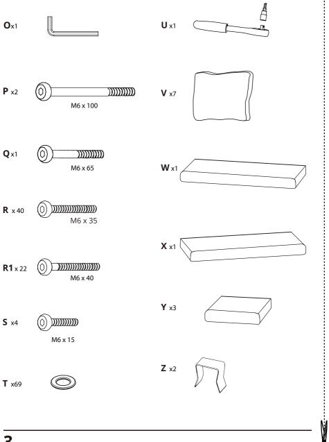
Please note, When building this product bolts should be finger tightened until all parts are in place. Only once all parts and bolts are assembled should bolts them be fully tightened using the ratchet.
