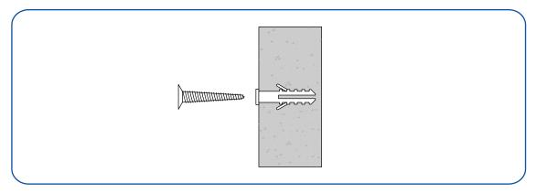
b. For Drywall or Hollow Walls: Ensure Phillips flat-head screws are anchored to studs, headers, or other structural wall components.
