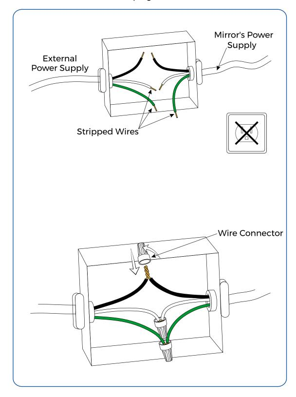
17. **Prepare Wires:** Strip the wires to the appropriate length. Ensure that the hardwires are not connected to a plug and socket outlet.
