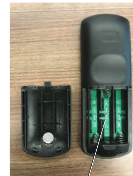
Polarity Markings Inside the Battery Compartment
