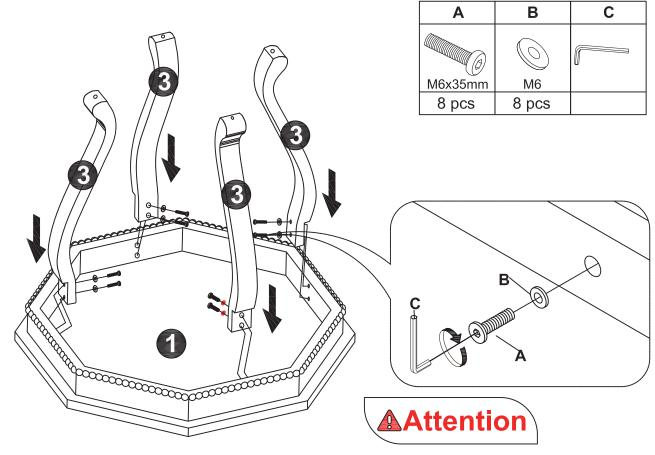
Initially tighten screws only halfway; do not fully tighten.
