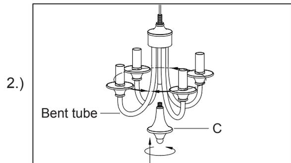
Step2: Rotate the bent tube to the suitable position. Screw the Decorating part (C) into the tube.
