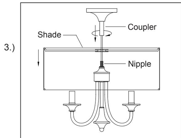
Step3: Place shade on the Nipple and tighten with the Coupler.
