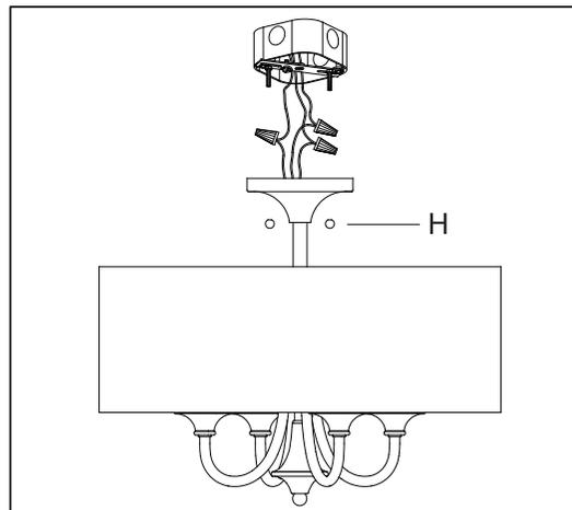
Step4.1: Wire fixture to wires in outlet box. Copper wire is for Ground. Attach canopy to mounting bracket and tighten with ball nuts.
