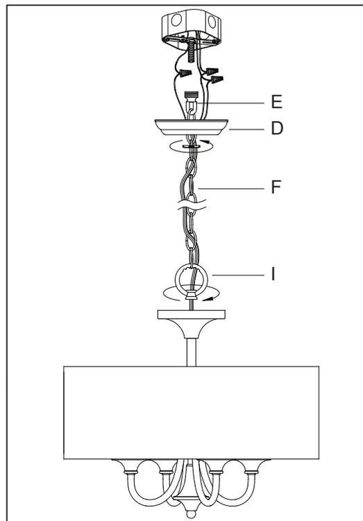
Step4.2: Install top loop to center stem and attach appropriate amount of chain to loop to achieve desired mounting height. Thread wire through every 3rd loop of chain. Remove ring from loop and slide down chain. Place canopy onto chain and let slide to top of fixture. Install nipple and cross bar into top of chain loop. Wire fixture to wires in outlet box. Copper wire is for Ground. Pull canopy through screw ring up chain to ceiling and tighten securely.
