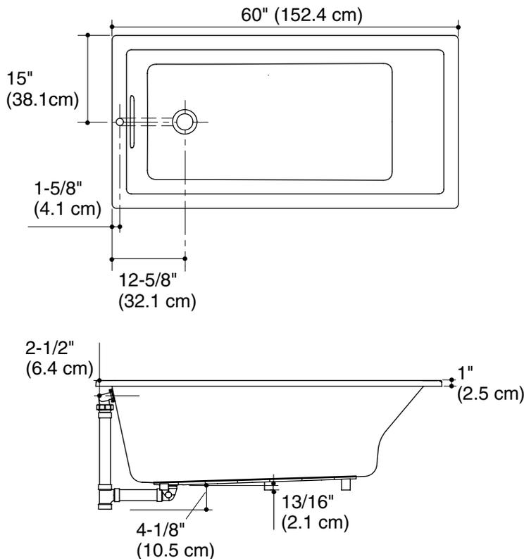
No change in measurement if connected with drain illustrated. (K-7272)
