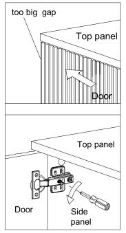
Turn the screw clockwise a little as shown to make the gap small.
