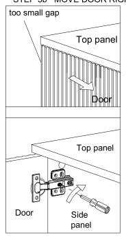
Turn the screw counterclockwise a little as shown to make the gap big.
