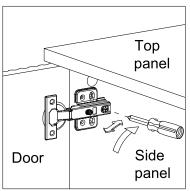
Loosen the screw indicated a little, adjust the hinge to right position (see step 2a & 2b), then tighten the screw.
