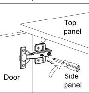
Loosen or tighten the screw indicated a little to adjust the gap between the door panels, adjust the hinge to right position (see step 3a & 3b).
