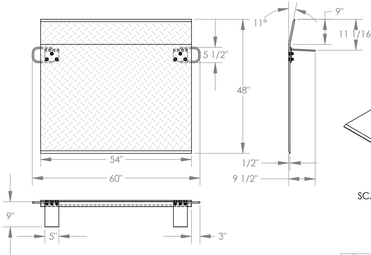
NOTE: BEND OR CROWN IS 11° AND LOCATED 9" FROM EDGE OF DOCKPLATE
