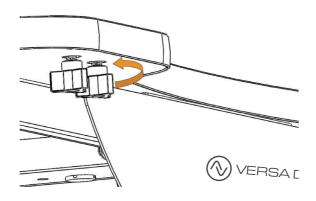
Pick up the keyboard surface. Align the slots on the side brackets to meet the loosened thumb screws on both the left and right sides. Gently slide the keyboard tray brackets into the gap between the thumb screws and the top surface.
