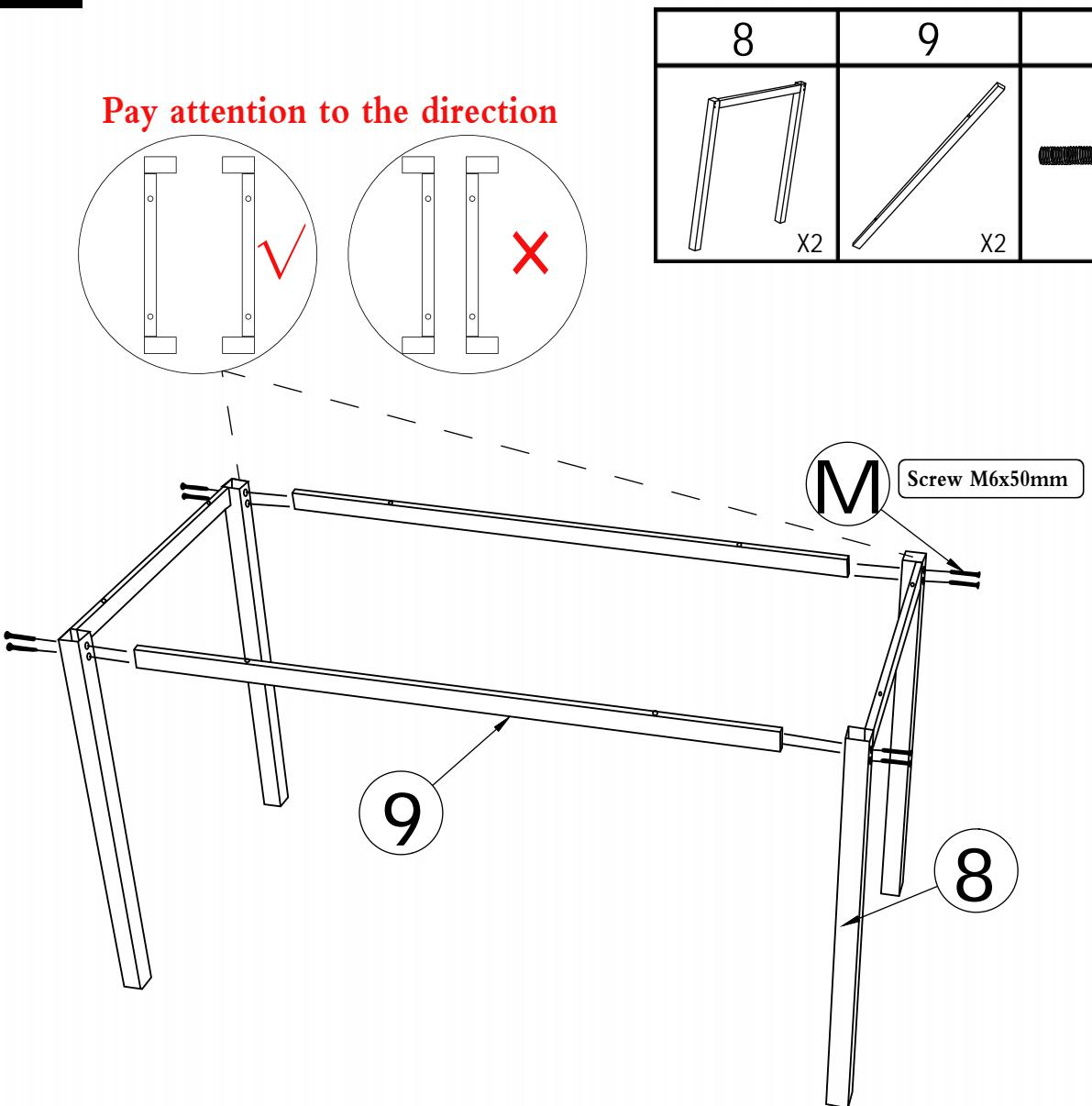
EN-During the assembly, please first half-tighten all the screws into the holes.
