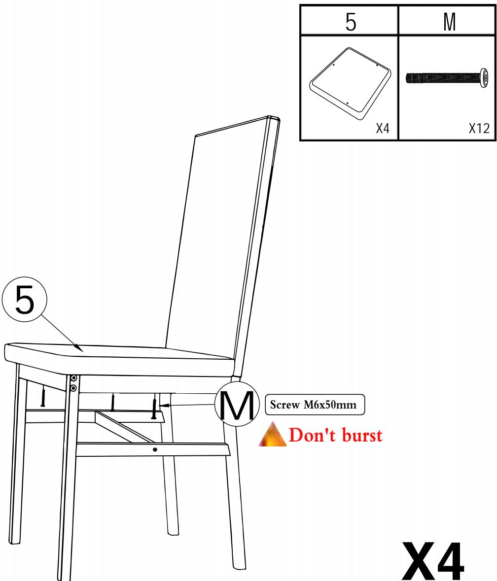
EN-During the assembly, please first half-tighten all the screws into the holes.
