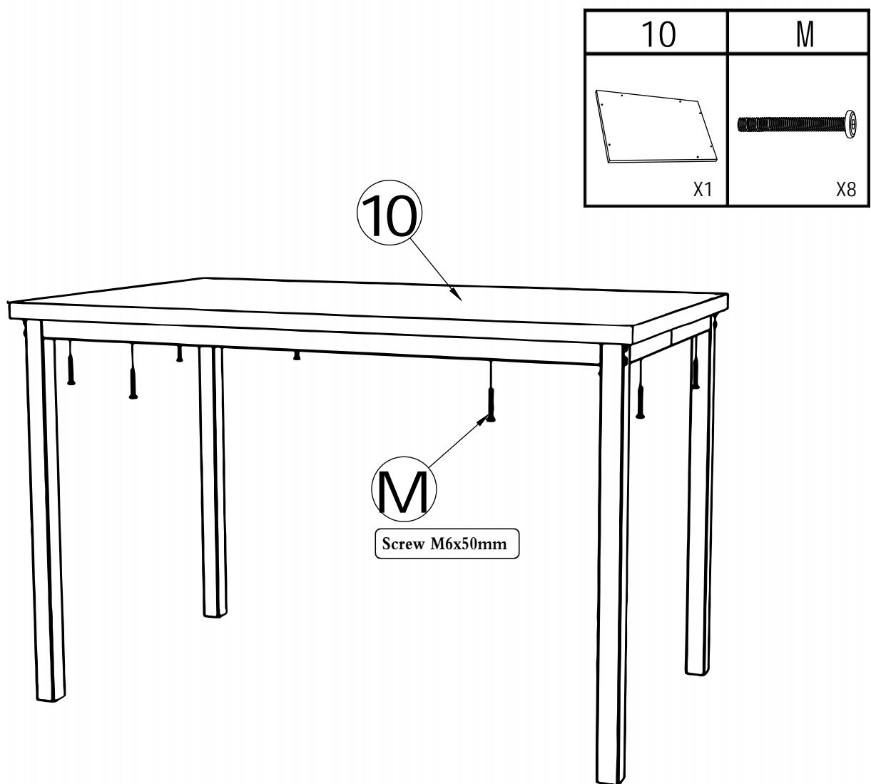
EN-During the assembly, please first half-tighten all the screws into the holes.
