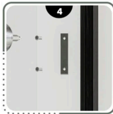
Match the magnet box well and screw in two metal plates.
