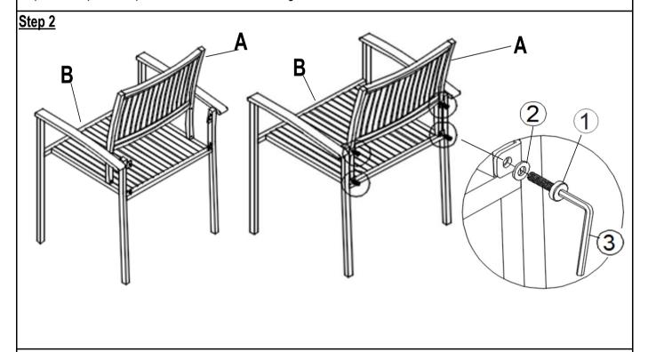
Attach Backrest Panel(A) to Seat Panel(B), secure using Bolts (1) and Washer (2) with Allen Key (3) as shown above .
