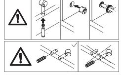
Insert the dowel (C) into the connection between components 6, 8, 11, 9, and 13 using the cam lock (B), turning the cam lock clockwise to tighten.
