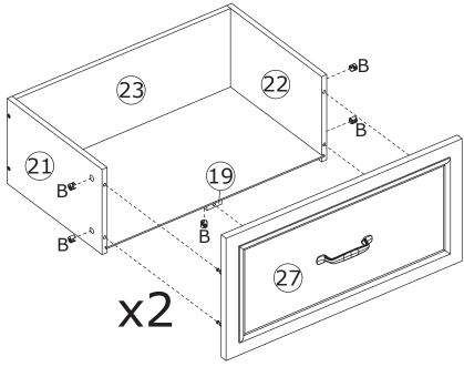
Connect components 19, 21, and 22 to components 27 and 28 using the cam lock (B), turning the cam lock clockwise to tighten.
