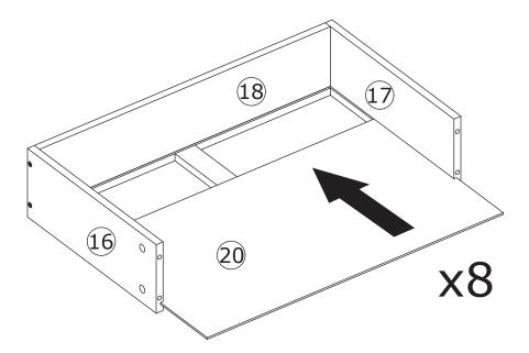
Insert component 20 into the available slot.
