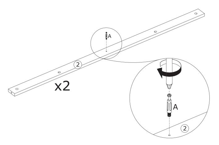
Insert the quick-install screw (A) into components 2 and 3.
