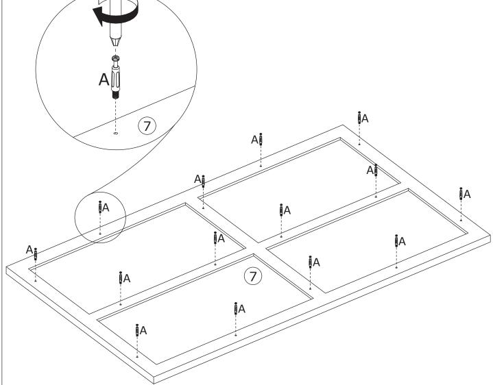
Insert the quick-install screw (A) into component 7.
