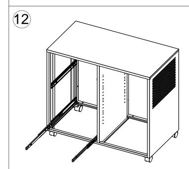
Pull out the small rails in the slide rails on the side walls completely.
