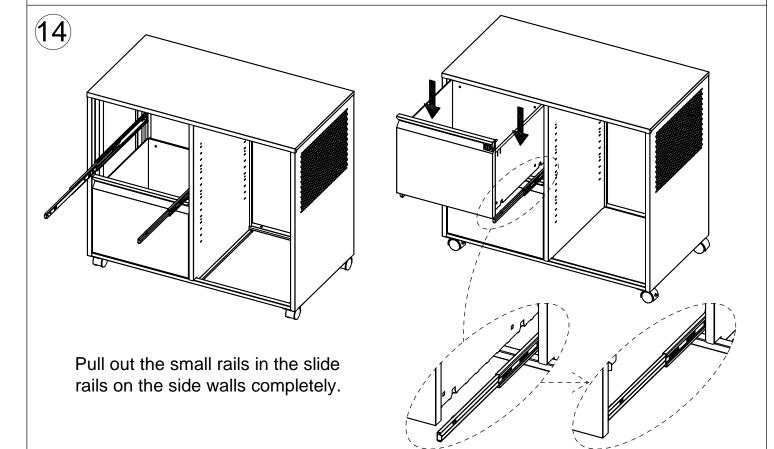
With two people lifting each side of the drawer, align the four divots on the bottom with the two rail clips on the rails on each side and insert them into the rail clips.
