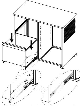
With two people lifting each side of the drawer, align the four divots on the bottom with the two rail clips on the rails on each side and insert them into the rail clips.
