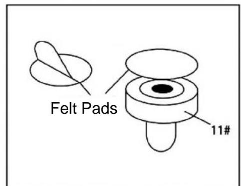
Tear the paper backing off the Felt Pads and stick them to the bottom of the Pushers (#11).
