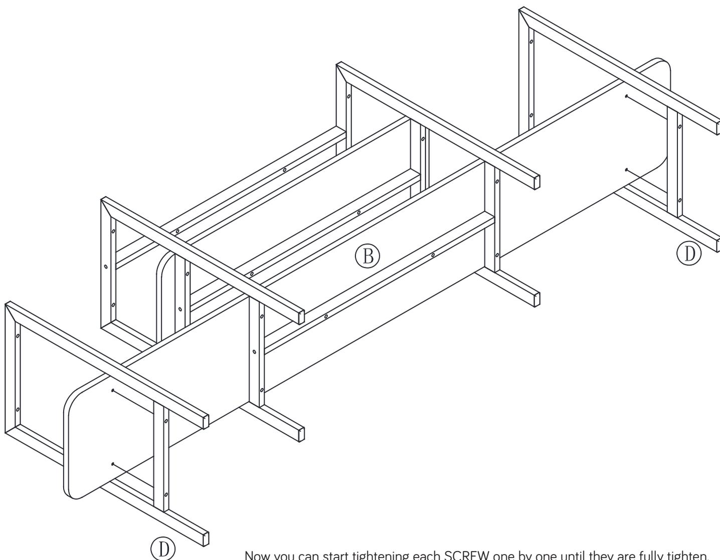
Now you can start tightening each SCREW one by one until they are fully tighten.
