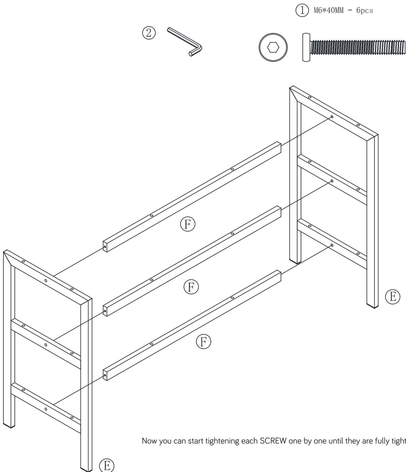
Now you can start tightening each SCREW one by one until they are fully tighten.
