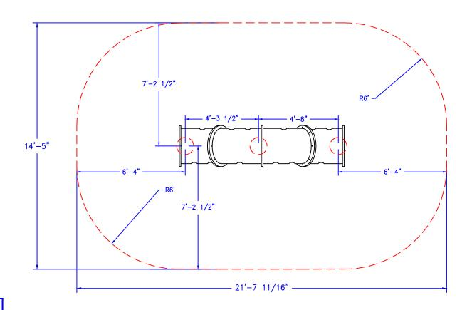
FOOTING DEPTH IS MEASURED FROM TOP OF SAFETY SURFACE. DEPTH IS 30" UNLESS NOTED OTHERWISE (SEE FOOTING DET.)
