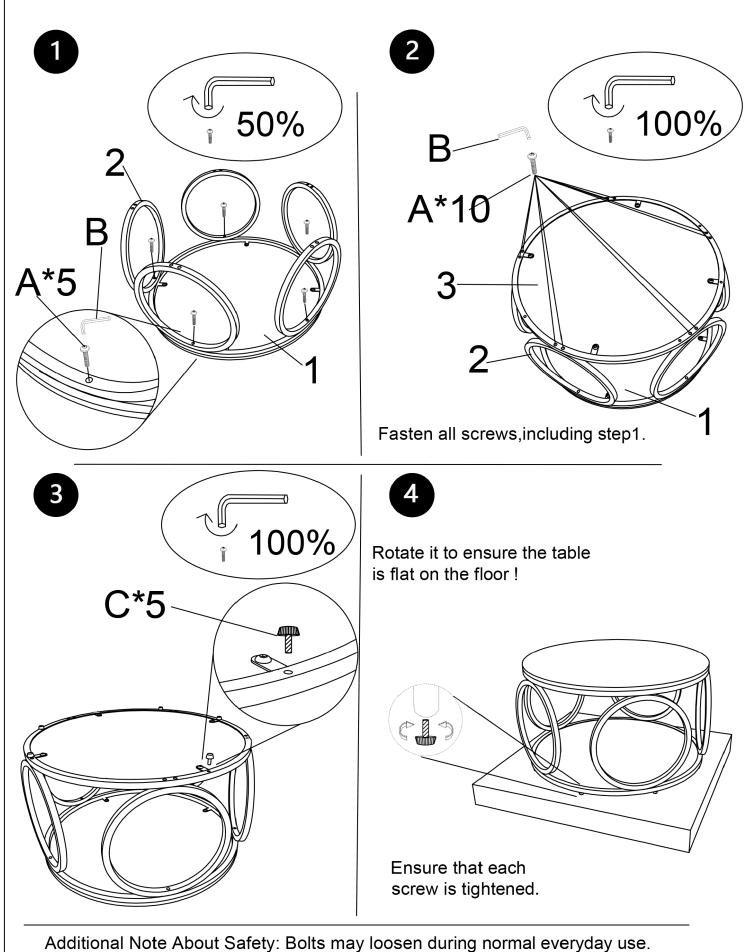
They should be periodically inspected and tightened to prevent damage or injury. Always check to be sure that all hardware is kept tightened.
