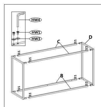
Step 1: Put the Flat washer(HW3) on the Hex bolt(HW1), insert the Crossbeam(B and C) into Leg frame(D) in order. Insert the Hex bolts into the mounting position and tighten them by using Allen key(HW4).
