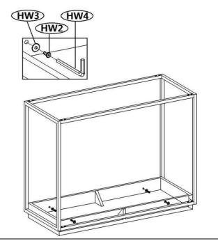
Step 3: Put the Flat washer(HW3) on Hex bolt(HW2), insert them into the mounting positions on the Table top(A), tighten then by using Allen key(HW4).
