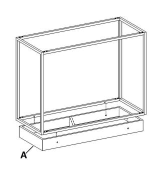
Step 2: Put the Leg frame on Table Top(A), make the mounting positions aligned.
