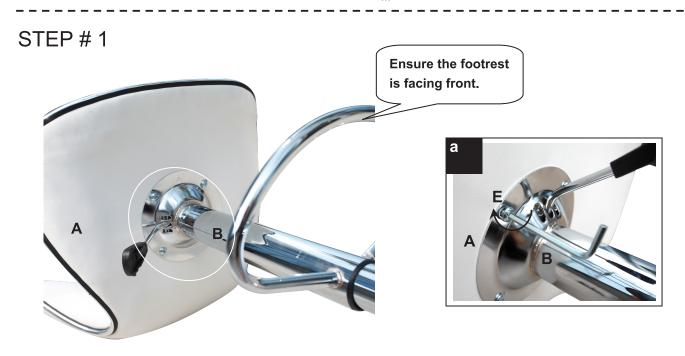
1. Attach steel seat plate (B) to the seat cushion (A) using four bolts (E) as instruction (a). Tighten the bolts with allen wrench
