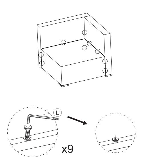
NOTE:IF ANY SCREW HOLES CANNOT BE ALIGNED, LOOSEN ALL THE SCREWS AND GO BACK STEP 1 AND RESTART ASSEMBLY.
