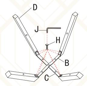
Twist Screw (H) to the (D) with (B) and (C).
