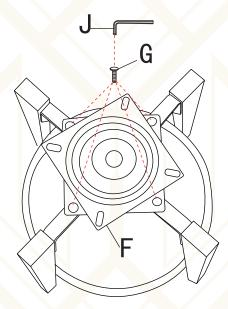
Rotate (F) 45 ° as displayed. Twist Screw (G) to the (F) with (B) and (C).
