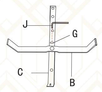
Place (B) on (C) as displayed, then twist Screw (G) to connect them. Only twist (G) into half way.
