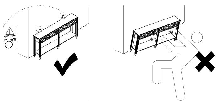
( Install tip-over restraint provided)
