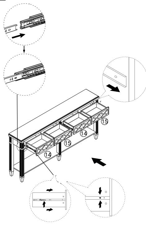
Please pull the movable silver component to the outermost part before inserting the pre-assembled drawer.
