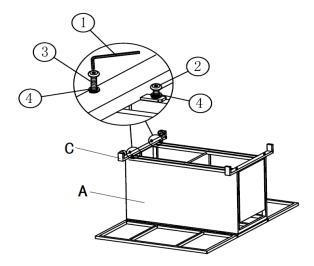
Align Table Leg with Wheels(C) to Table Body(A) and attach using Bolts(2), Bolts(3) and Washers(4) with Allen Key(1) as shown in the picture.
