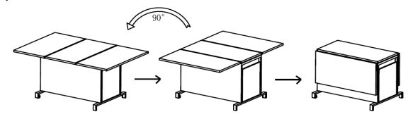
**To close the Table Top:** Unclip the Table Top from the Metal Bars, then rotate the Table Top back 90 degrees.
