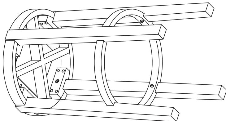
Do not tighten bolts completely until all bolts are completely lined up and inserted into holes.
