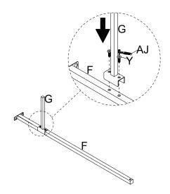
Attach the Center Rail - Front / Rear (F) to the Headboard (A) and the Footboard (B), insert the Bolt (Y), turn the Ratchet Tool (AJ) to tighten them. Then attach the Center Rail - Front / Rear (F) to the Center Support Bar (C), insert the Bolt (Z), turn the Ratchet Tool (AJ) to tighten
