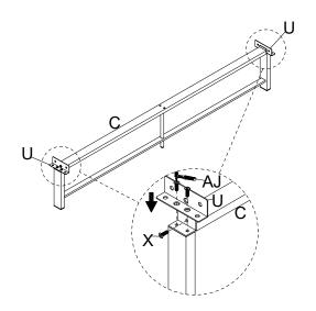
Attach the Bracket (U) to the Rail Section - Front (D) and Rail Section - Rear (E), insert the Bolt (Y), turn the Ratchet Tool (AJ) to tighten them.
