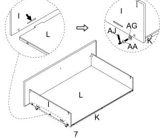
Attach the Drawer Back Board (J) to the Drawer Bottom Frame (K), insert the Bolt (AA) and Washer (AG), turn the Ratchet Tool (AJ) to tighten them. Attach the Drawer Board Connector (Q) to the assembled drawer, insert them into correct places.
