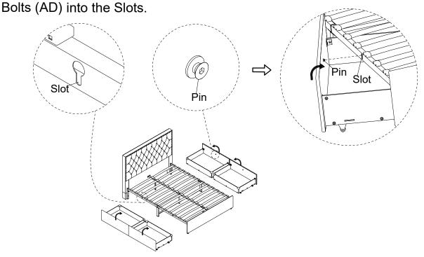
When pull out the drawers, lift the drawers first in order to make the Pins released from the Slots freely, then pull the drawers toward outside. DO NOT PULL OUT THE DRAWERS DIRECTLY.
