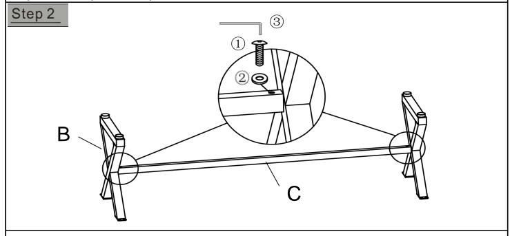
Attach Leg with pre-attached Levellers(B) and Leg Support(C) with Bolts(1) and Washers(2) by Allen Wrench(3).
