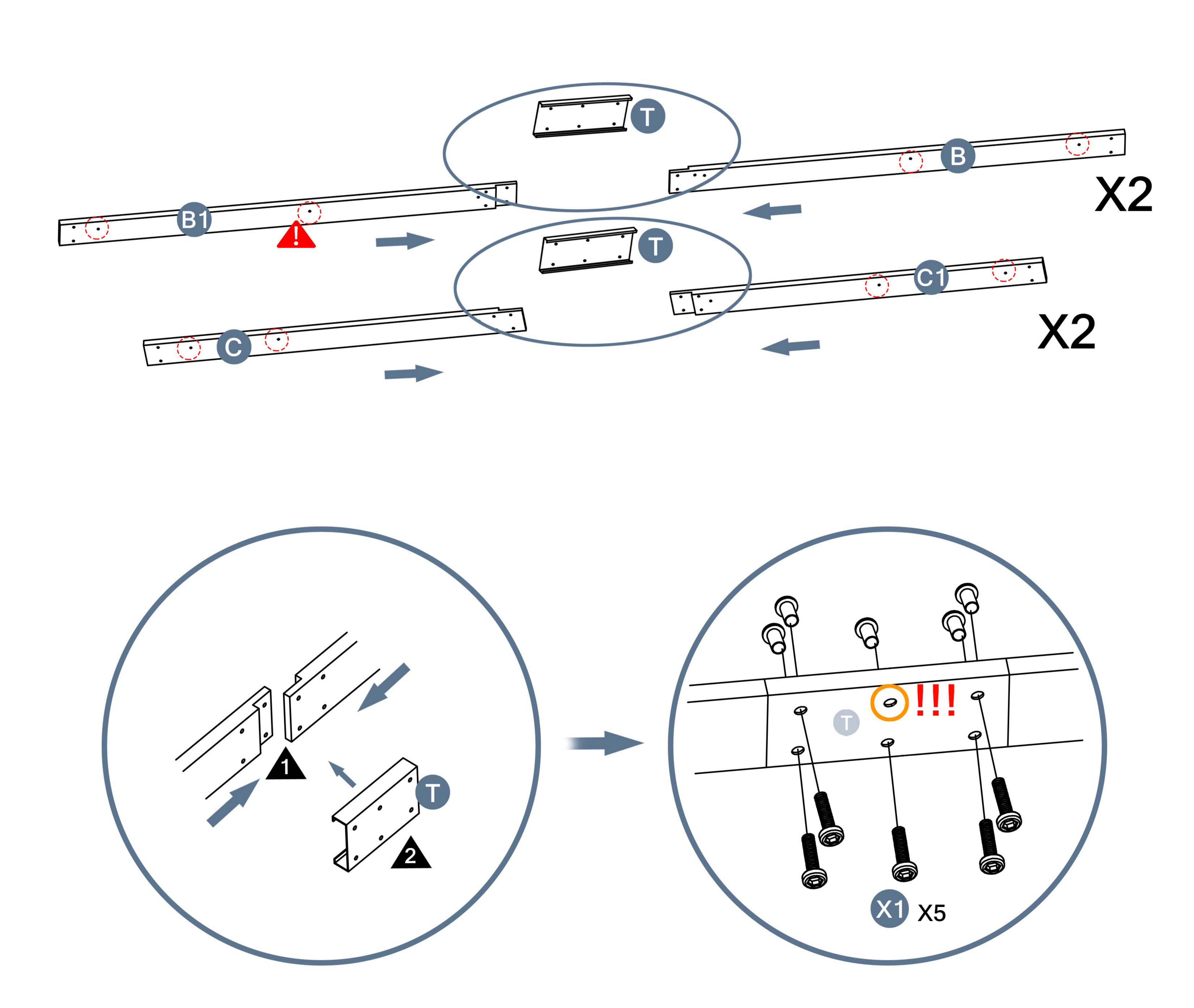
Be careful not to screw the screws at the yellow circle. Step 6 is screwing.
