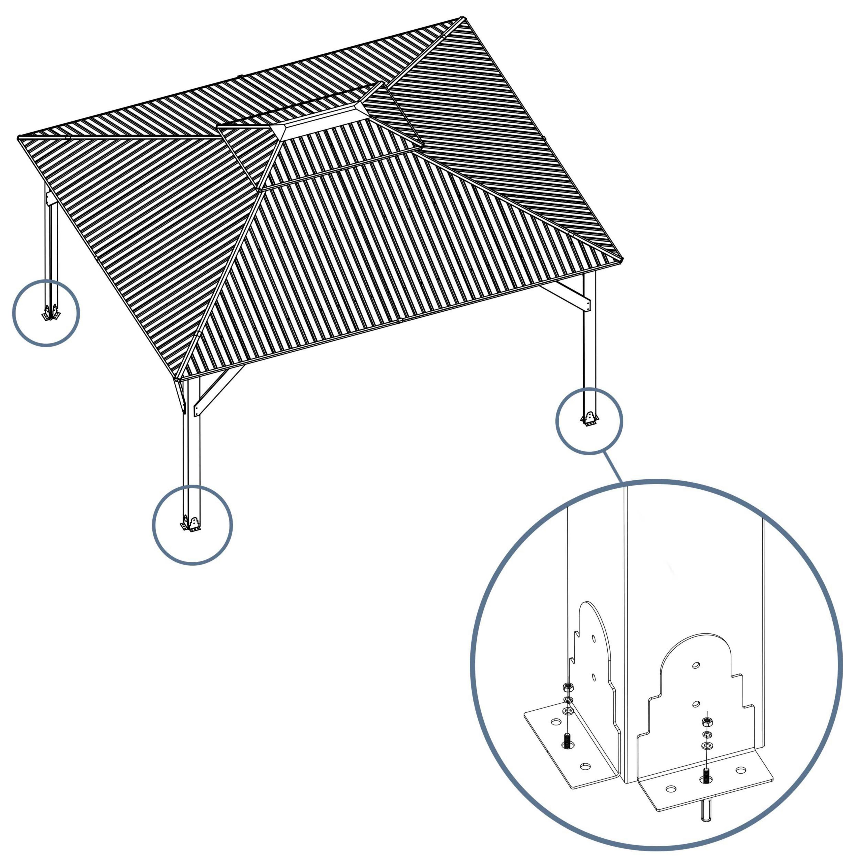
For safety's stake, please check and make sure that all screws are tightened after all installation is complete.
