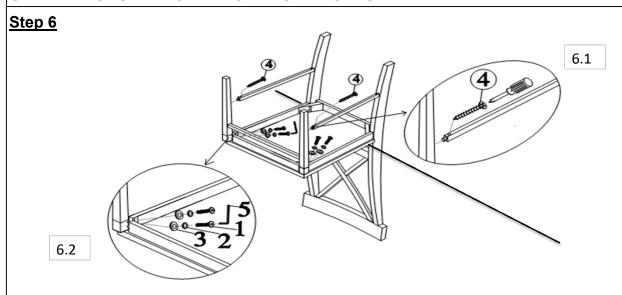
Place complete part in step 2 into the tenon of sail rails and the Chair Seat (B).
