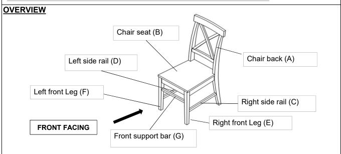
This Chair has multiple parts and may require up to some 30 minutes to assemble. To give you an overview of the Chair, the above picture is to assemble is to help you put the various parts into perspective. Please read through the instructions here below to familiarise the parts and steps before assembly.
