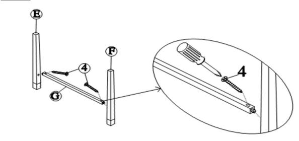
Attach Front support bar (G) into the upper housing of the Top Right Front Leg (E) and Top Left Front Leg (F).
