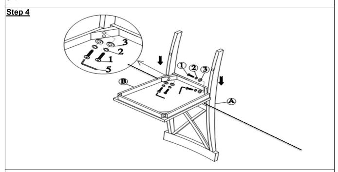
Secure the Chair Back (A) to the Chair Seat (B) by using Bolts (1), Spring Washer (2), Flat Washer (3) and Allen Key (5).
