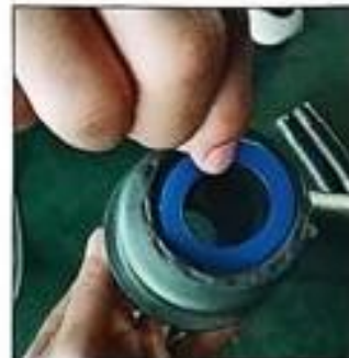
10: Put the sealing ring on this pipe joint
