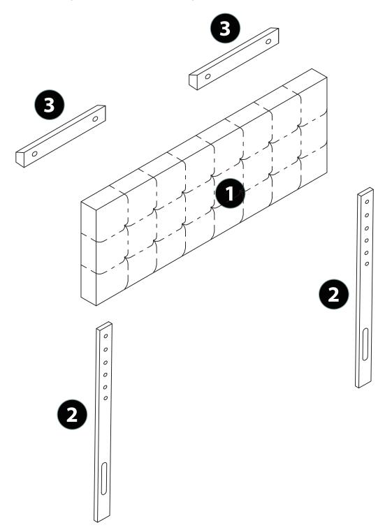
This drawing is to give you an overall idea only of how this assembly will go together and does not replace the assembly instructions.
