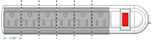
Adapter must be 1.1" wide or less to fit side by side on power strip.
