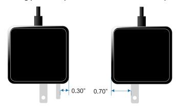
For power adapters with the grounding pin, measure from the edge of the adapter closest to the grounding pin. This dimensions must be 0.30" or less to fit on the 10 outlet power strip.
