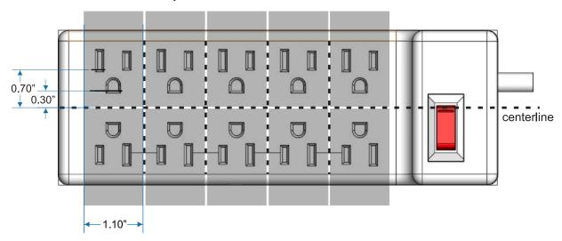
Adapter must be 1.1" wide or less to fit side by side on power strip.
