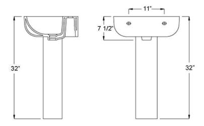
Dimensions of fixture are nominal and may vary within the range of tolerances established by ASME Standard A112.19.2-2008. Dimensions and specifications subject to change without notice.
