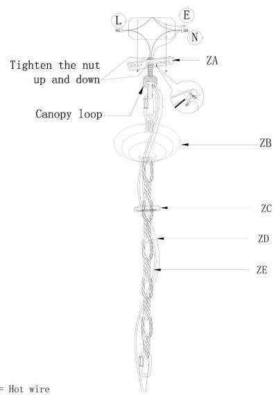
IMPORTANT: Test sockets with bulb before dressing the fixture.
