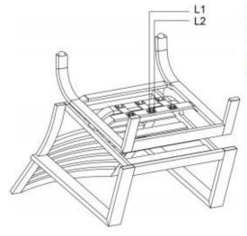
Use wrench (J) and wrench (K) to secure the nut and bolt in location (L1) and location (L2). See below diagram.
