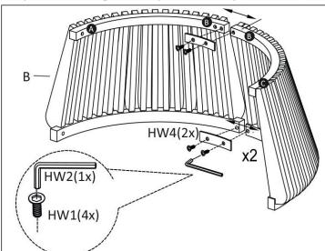
**STEP 1:** Position base segments like this & match the characters marked on each to make a series. Place the assembly plates & tighten the bolts as shown above.
