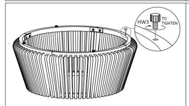
**STEP 4:** Place the base ring upside down and carefully tighten the levelers as shown above.
