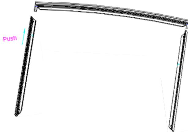
2. After making sure that all four corners join at right angles (forming a perfect rectangle), fasten the four angles together by using x8 **M5 screws (E)**.
