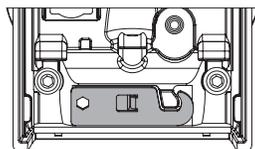
Insert spray removal tool into spray slot by sliding hook end of key between faucet spout and insert. Pull insert out of faucet once hooked.
