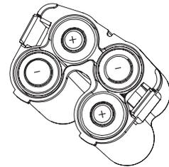
Replace cover of the battery pack assembly and reinsert assembly into faucet.
