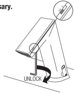
Remove battery pack assembly by lifting out of spout.
