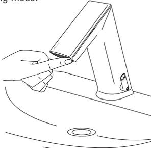
Cover IR clic until LED flashes 4x - hold on until LED flashes 1x to 8x, from minimum to maximum. See diagram below. Release when requested range is reached.
