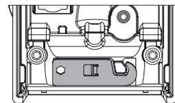
**NOTE: If spray head is inserted incorrectly – key will not lock in properly. Turn faucet on to push insert out and re-install.**
