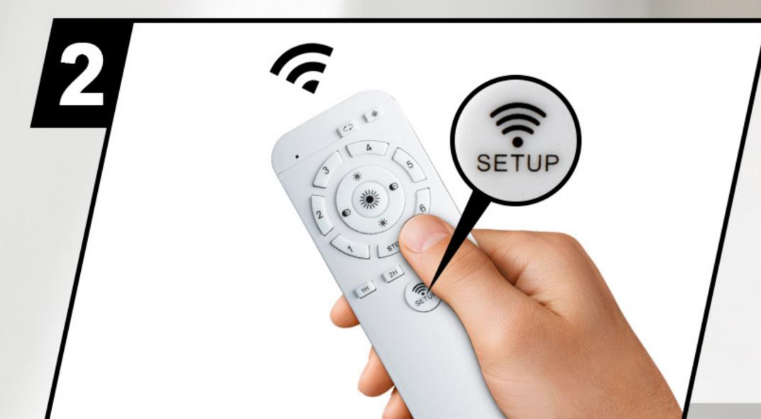
Press the STEUP button on the remote to reconnect.
