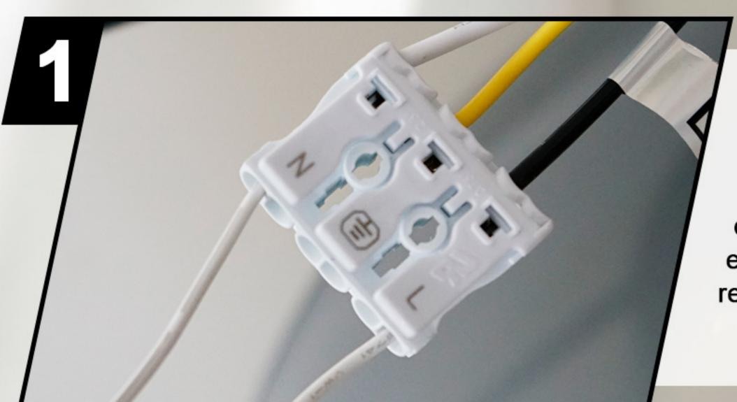
Before connecting the new remote control, it is necessary to disconnect the zero and live wires before reconnecting them. This is to clear the data left by the previous remote control and enable the fan to obtain data from the new remote control.
