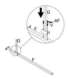
Attach the Center Rail - Front / Rear (F) to the Headboard (A) and the Footboard (B), insert the Bolt (V), turn the Ratchet Tool (AF) to tighten them. Then attach the Center Rail - Front / Rear (F) to the Center Support Bar (C), insert the Bolt (W), turn the Ratchet Tool (AF) to tighten
