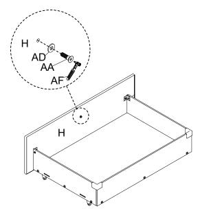
Align drawers with the bed frame and push them into the bed. Lock drawers by slightly lifting drawers and inserting the Pins that the heads of Bolts (AA) into the Slots.
