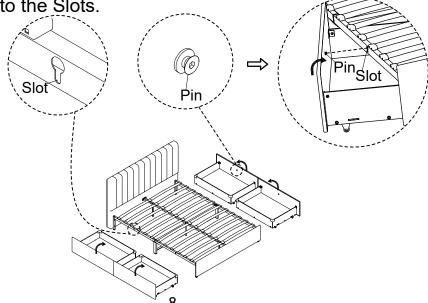
When pull out the drawers, lift the drawers first in order to make the Pins released from the Slots freely, then pull the drawers toward outside. DO NOT PULL OUT THE DRAWERS DIRECTLY.
