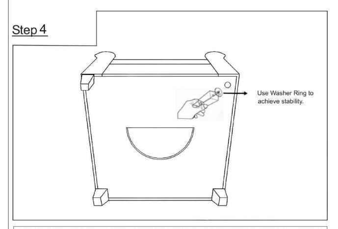
Install the leg into the chair by putting a Washer Ring (optional) on the threaded stem and then insert the threaded stem into the threaded hole at each corner of the bottom of the chair. Tighten by turning leg clockwise. Repeat the same procedure to install the other 3 remaining legs.
