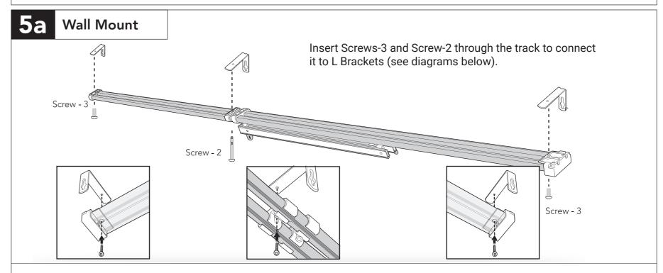
Position the track to where you would like to hang it on the wall (using a level is recommended). Mark the screw position of the L Brackets (use the top tip of the L bracket opening, as that is where the track will hang from).
