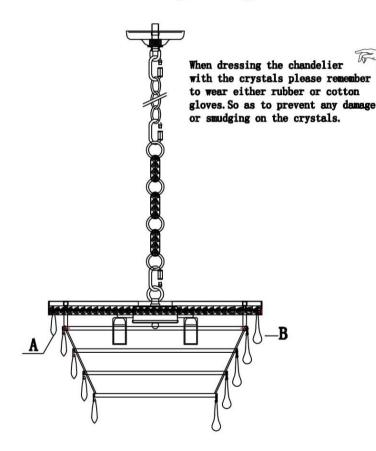
1. Hang the crystal (A) and the crystal (B) on the first circle to the fifth circle of the Lamp Frame as shown in the figure.
