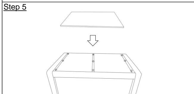
Place the Glass Top(D) on the assembled Table Frame.
