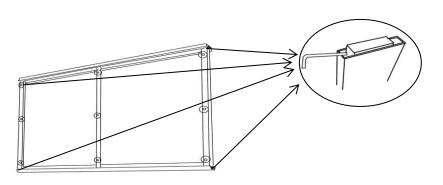
Take out the silders in the four ends of Table Top Frame(C) using Allen Key(③).
