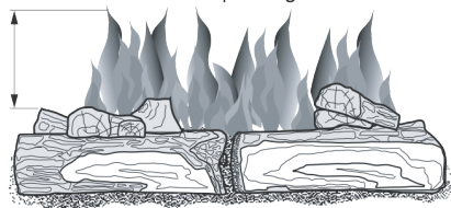
Figure 20 - Incorrect Burner Flame Pattern
